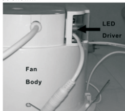
Diagram 3 Connect connector to the LED driver
